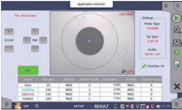
MT1000A screen displays details of the fiber tip core, cladding, adhesive and contact, with automatic Pass/Fail result judgement.
